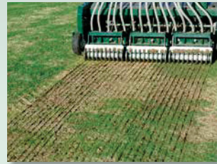
TriWave technology creates the optimum slits for improved seed-to-soil contact, while minimizing turf disruption.
