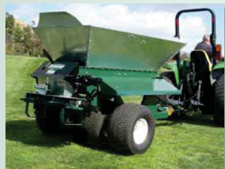
Four-wheel walking beam suspension.
