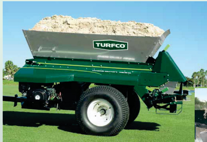
Redesigned hopper has 20 percent greater capacity and the widest opening in the industry, so you'll refill faster and spill a lot less.
