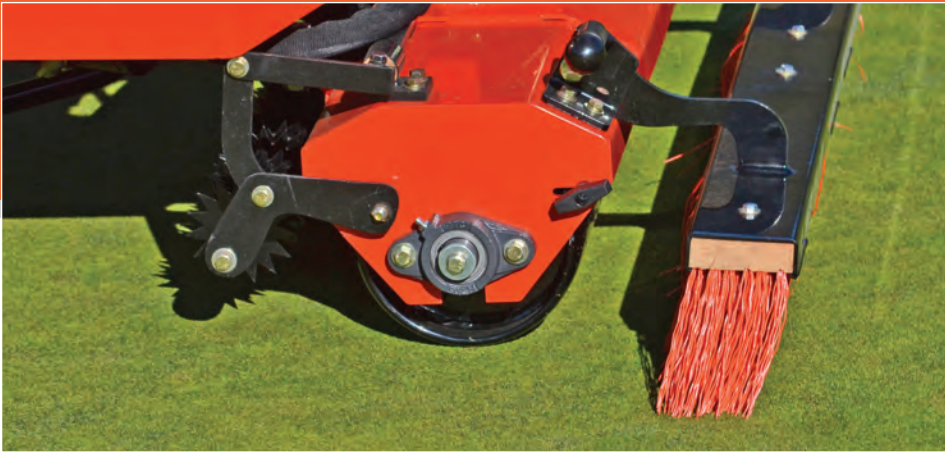
Model 7580/7590 equipped with Model 7512 Spiker Attachment & 7514 Brush for even better greens health and playability
