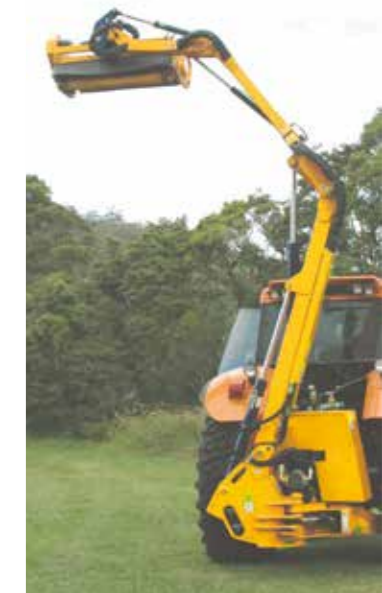
Reach great heights With forward positioning and two reach options of 7.1m and 8.0m.
