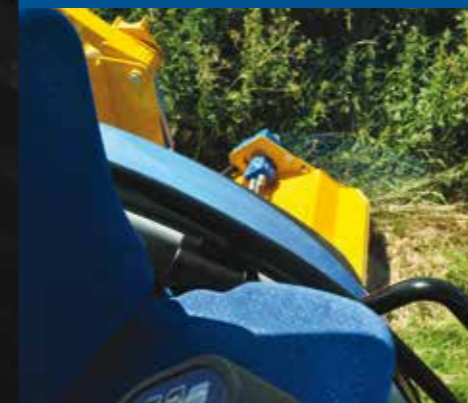
Clear visibility Variable forward reach brings cutting head into drivers view.
