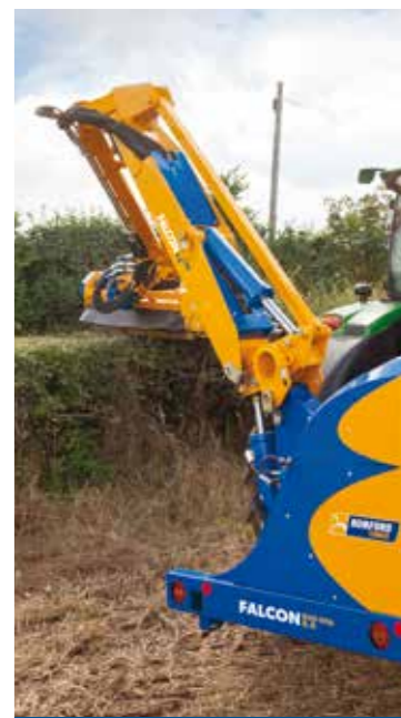
Variable Forward Arm The VFA allows total flexibility of position during arms operation.
