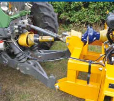
Fitting kits for tractor front linkages Options for 1000/540 RPM.
