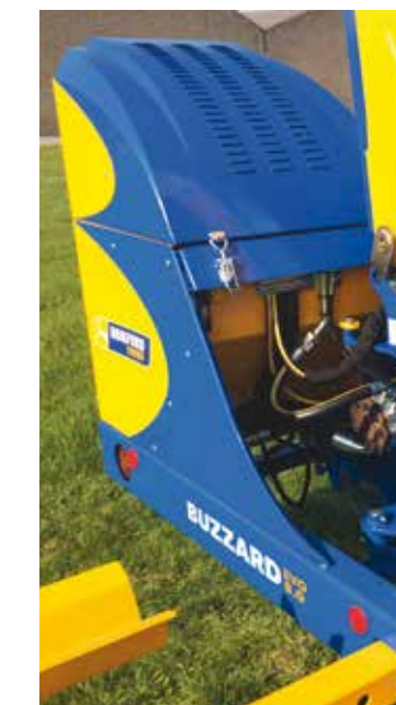
Fully enclosed hydraulics Keeping components protected from the elements.
