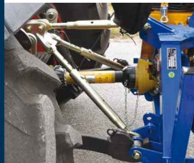
SYSTEM 1: THREE POINT LINKAGE
